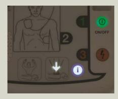
**If a shock has been delivered**,he i button will flash blue and can be pressed for CPR voice prompt.
