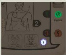
If no shock is advised even if you press the orange shock button, there is no way the device can deliver a shock.
